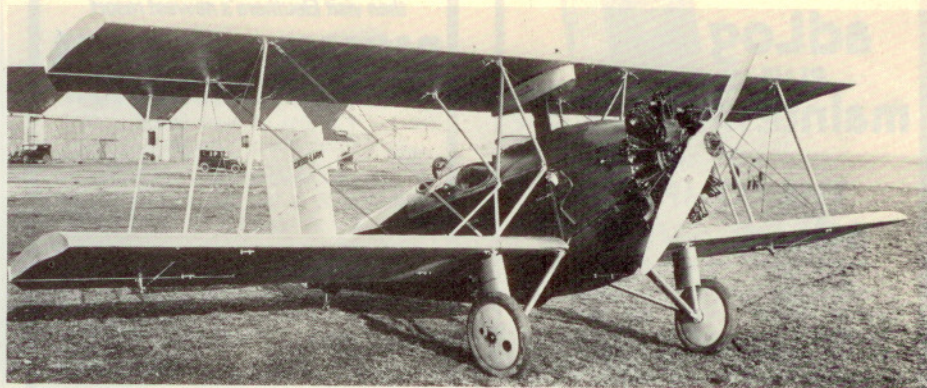
The final version of the Lark had the 200-hp Wright J-4 Whirlwind engine. Note the auxiliary fuel tank under the upper wing and the faired-in belly cargo container. The bent metal propellers shown in all of the photos were developed by Dr. Sylvanus Albert Reed under Curtiss sponsorship and were manufactured and sold by Curtiss as the Curtiss-Reed propeller into the 1940s.
