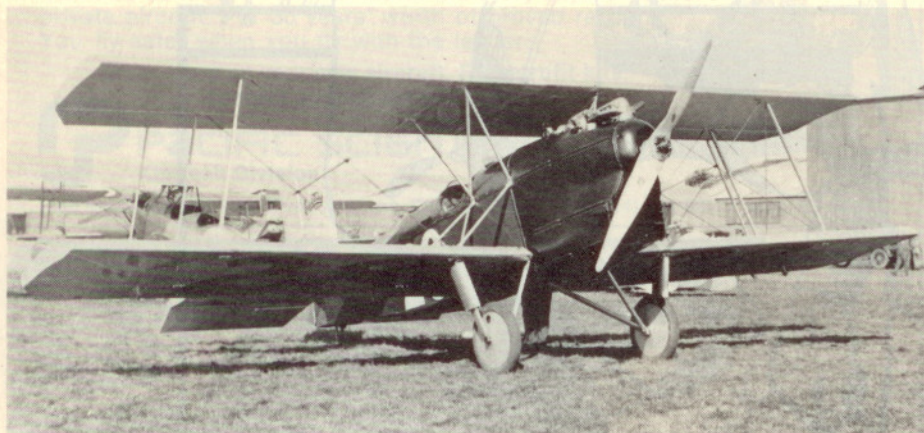
The prototype Curtiss Lark with C-6 engine and 1925 National Air Race numbers. Note that the shock absorbers on the landing gear are installed outboard of the wheels.
