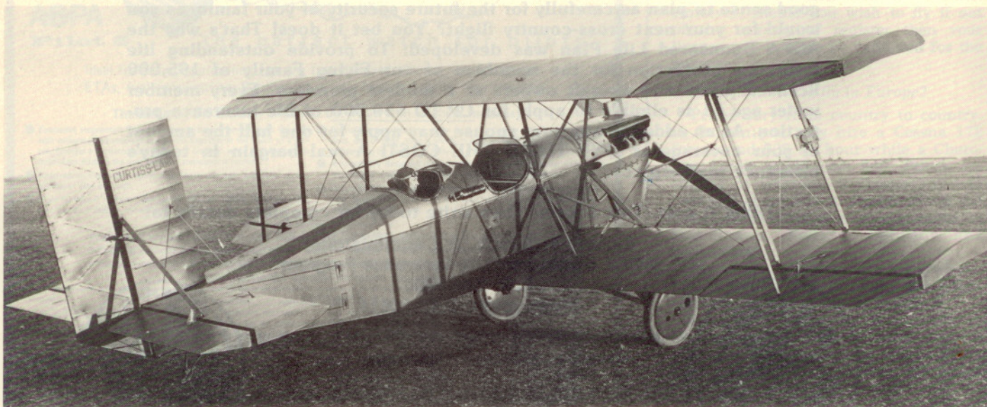
Three-quarter rear view emphasizes the angularity of the Lark. This is the second article, with a 180-hp "Hisso" engine and three-seat configuration with the pilot alone in a smaller, rear cockpit. The landing gear has widened and the shock absorbers are now inboard of the wheels.
